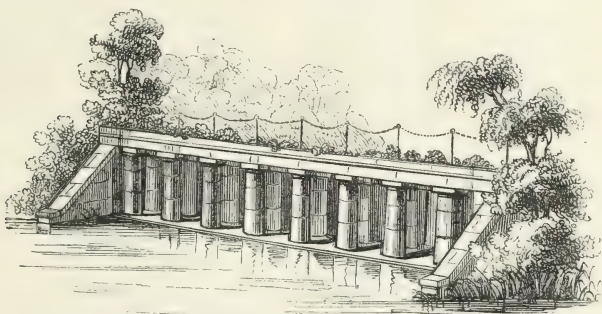
[Fig. 222. Viaduct proposed for Woburn Abbey, in order to disguise the dam, or head, which separates two pieces of water on different levels.]
